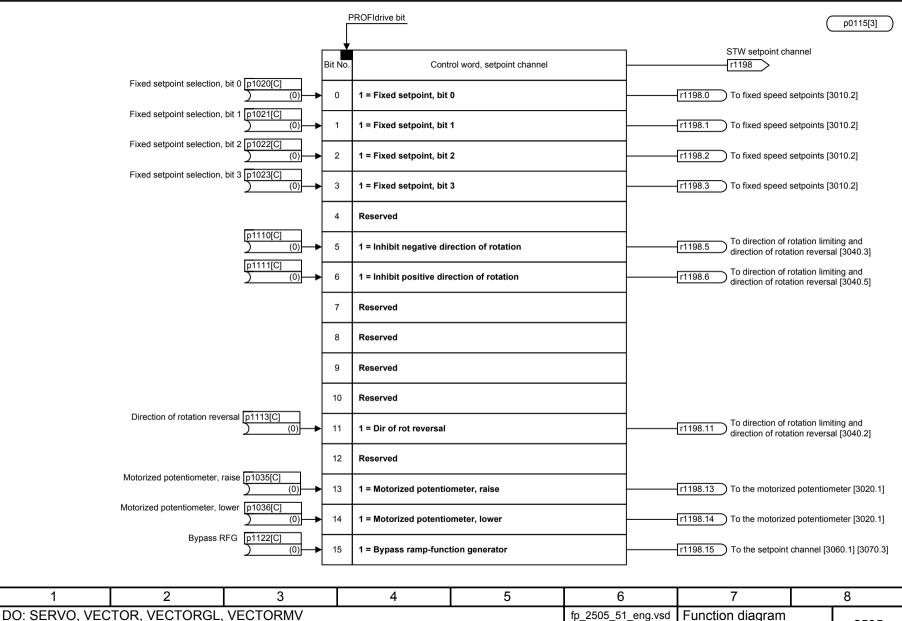
31.05.06 V02.05.00 SINAMICS Internal control/status words - Control word, setpoint channel
