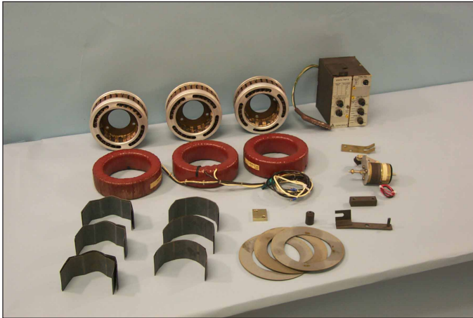
Fig. 1 Overview: Original Components Removed from the Breaker.
