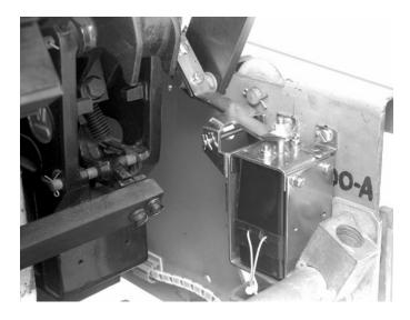
B. The DTA reset adjustment is achieved by turning the flange nut on top of the DTA shaft. If adjustment is required, remove the flange nut from the DTA shaft and apply Loc-Tite<sup>®</sup> 242 to the shaft threads. Then screw the nut onto the shaft, adjusting the gap to .19" - .25" as shown.
