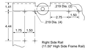
B. For Version "S" Breakers, use Drilling Plan C then drill and countersink two .281" diameter holes in both the right and left Breaker Frames. These holes will be used to mount the Trip Unit Mounting Platform and attached components later in the Retrofit process.
