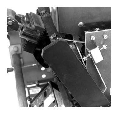
Step 12: Installing the Trip Finger Assembly
