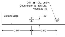
Right Side of Breaker Shown – Drill Both Sides (11.50" High Side Frame Rail)
