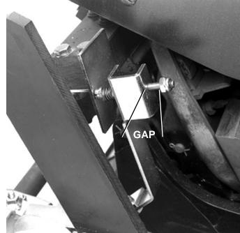
NOTE: To provide clearance for the Racking Mechanism Lock, the bottom front DTA Assembly mounting screw must be inserted with the screw head towards the outside of the Breaker.
