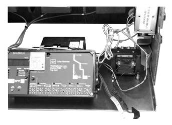
E. Attach the Glass Poly Insulation Plate to the top of the CPT, as shown, using the screws and lock washers supplied with the CPT kit.
