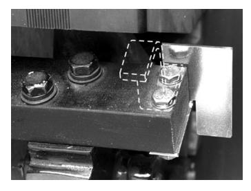
A. Align the holes in the DTA Mounting Brackets with the holes drilled in the right Breaker Frame in Step 8. Using the .190-32 × .625" screws, flat washers, lock washers, and nuts provided, mount the DTA Assembly to the right Breaker Frame as shown. When positioning the DTA Assembly, assure that the Reset Lever is behind the Striker Plate.
