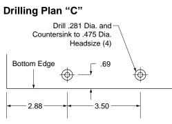
Right Side of Breaker Shown – Drill Both Sides (10.50" High Side Frame Rail)
