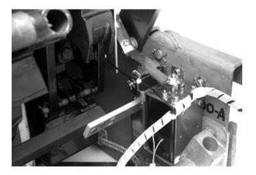
G. For Kits Supplied With An Auxiliary Switch Only. Route the two wires, with ring terminals, from the External Harness along the right side of the Breaker to the Microswitch Switch. Connect one wire to the normally "Open" terminal and the other wire to the "Common" terminal.
