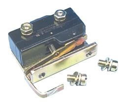
Align the Aux. Switch Assembly with the holes in the DTA Assembly. Secure the Aux. Switch Assembly to the DTA Assembly, as shown, using the (2) .190-32 x .375" screws, (2) flat washers, and (2) lock washers provided.
