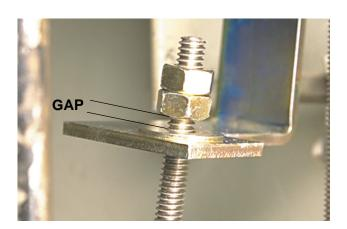
C. Back off the nuts on the bottom of the DTA Reset Assembly Shaft and apply Loc-Tite® 242 to the threads.
