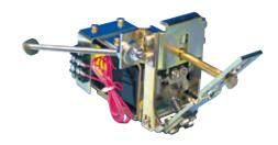
C. While holding the DTA Assembly near the holes drilled in the right Breaker Side Plate in Step 3-B, insert the Trip Link into the hole in the Trip Finger. Loosely install a .250" wide flat washer and two (2) .250-20 nuts.
