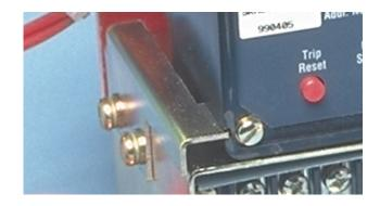
E. Fully tighten the 4.00" screws that secure the Trip Unit to the top of the Aux. CT Module.
