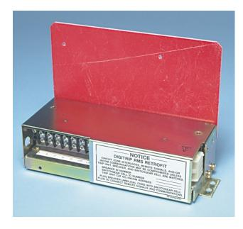
B. For Kits Supplied with a PT Module Only. Mount the PT Module to the Glass Poly Insulation Barrier, as shown, using the (2) .138-32 x .500" screws, (4) flat washers, (2) lock washers, and (2) nuts supplied.
