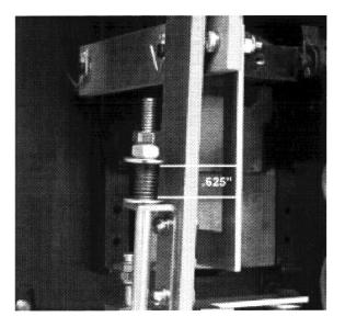
B. Measure the gap between the flat surface of the flange nut on the top of the DTA Shaft and the bottom surface of the Trip Arm. The gap should be .09 to .12". If the gap is not within this range, back off the flange nut and apply Loc-Tite® 242 to the threads of the DTA Shaft. Adjust the flange nut until the gap is within the acceptable range.
