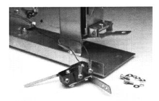
D. Mount the Auxiliary Switch Assembly to the Aux. CT Module Mounting Platform, as shown, using the (2) .164-32 x .500" screws, (4) flat washers, (2) lock washers, and (2) nuts supplied.
