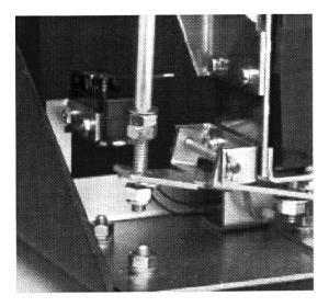
Align the Reset Assembly Pivot Bracket with the holes in the Connecting Link Bar. Secure the Pivot Bracket to the Connecting Link Bar, as shown, using the original hardware.
