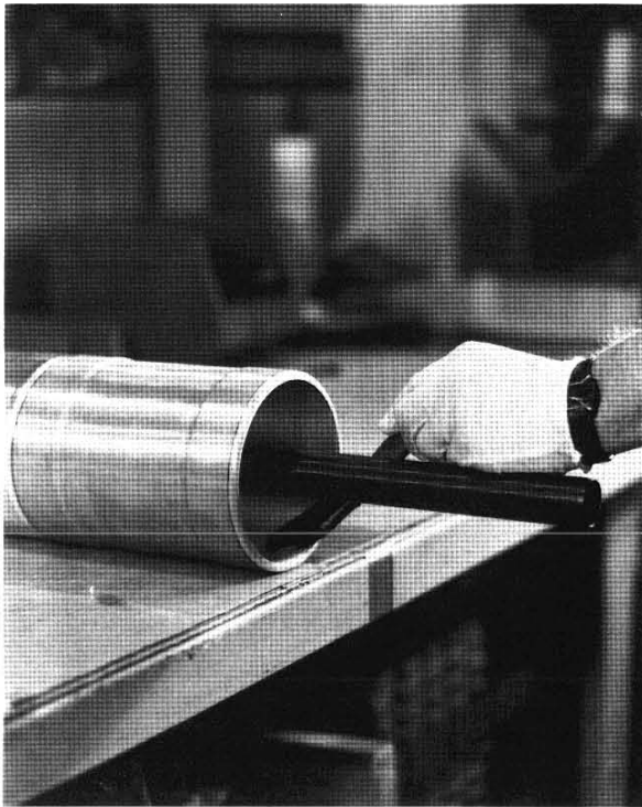
Plate 40: Placing the interrupter tube on the interrupter assembly fixture
