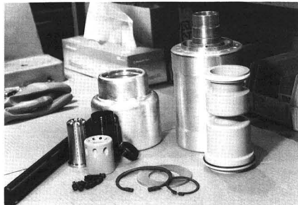
Plate 10: Components of the moving contact assembly
