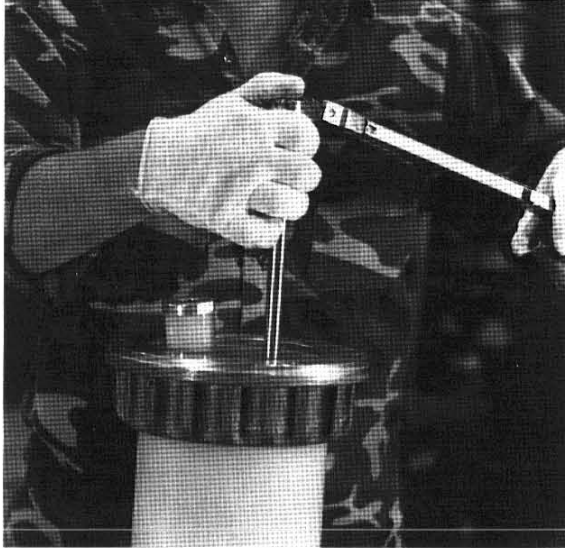
Plate 43: Re-installing the interrupter support tube
