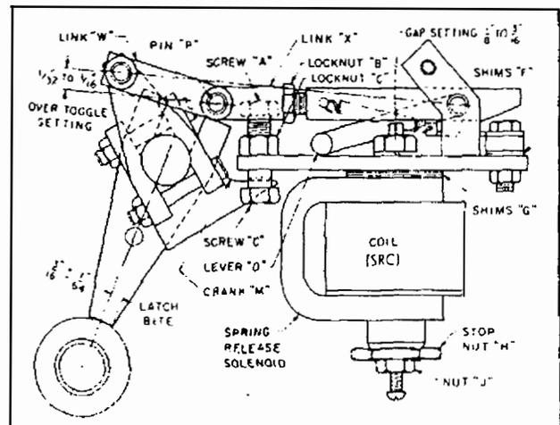
**Caution** - Over toggle linkage (W, X and Pin P) must be free to move through the toggle position with crank (M) against screw (A) without moving latch (18). Otherwise, excessive load may exceed the output of the spring release coil (50), preventing the breaker from closing.
