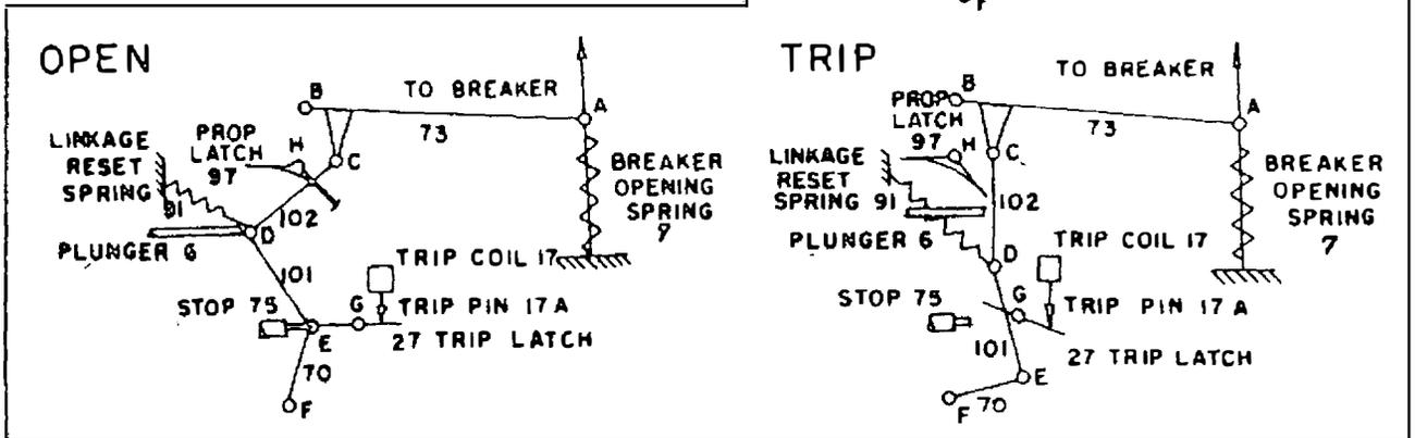
Fig. 5 - Type SE-3 stored energy operator.
