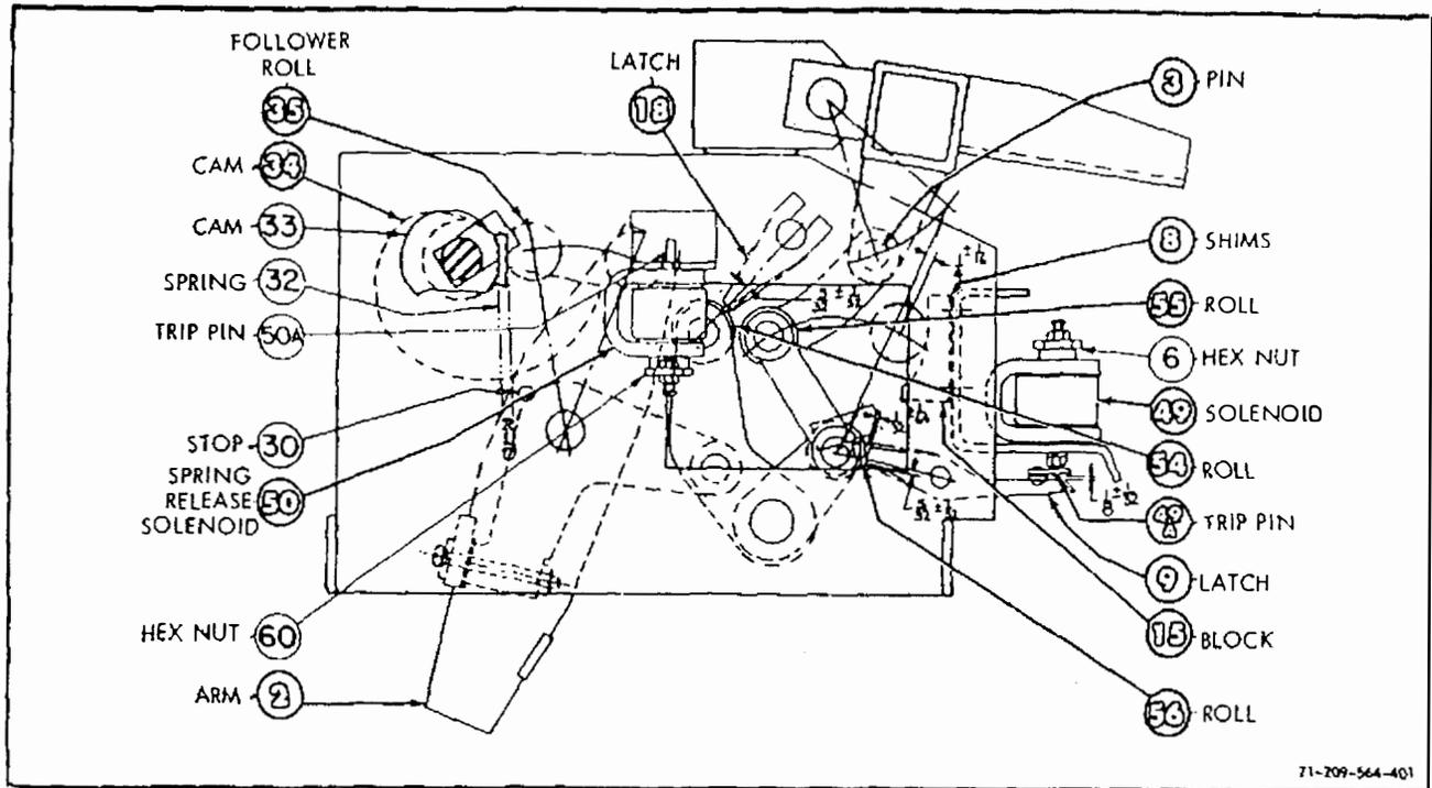
Fig. 19 - Type SE-3 stored energy operator assembly.
