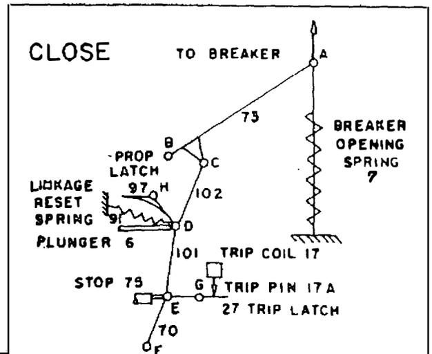
Fig. 4 - Four-bar linkage.
