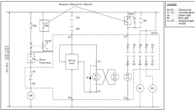
Figure 9 – Standard operation circuit of the latched type (shunt trip)
