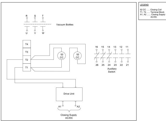
Figure 6 - Internal connection of the normally energized type
