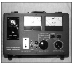
Figure 11 - Toshiba Portable Vacuum Checker
