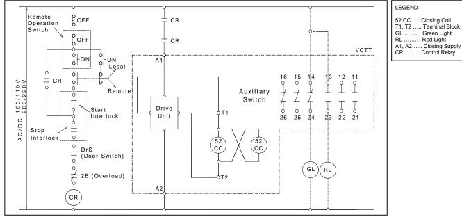
Figure 8 – Standard operation circuit of the normally energized type
