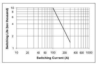
Figure 14 - Capacitor Switching Life
