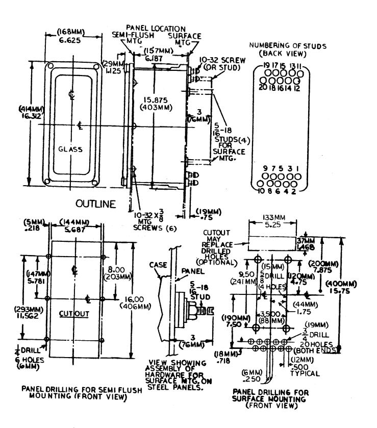
Fig. 2 (K-6209274-4) Outline and Panel Drilling Dimensions for an M2 Size Case
