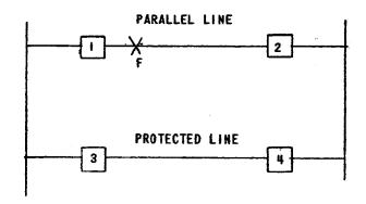
Fig. 4 (0246A3661-0) Typical Situation Leading to a Power Reversal in the Protected Line
