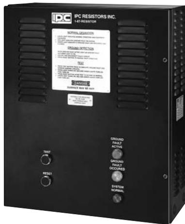
The **StopLight™** system uses a unique indicator light system to provide visual detection of a ground fault. A red signal indicates an active ground fault, an amber light indicates a ground fault has occurred and a green light signifies there are no active ground faults on the system.
