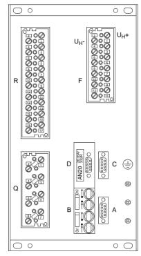
Figure 2-6 Rear view of a 7SA6, housing size 1/3 (terminal arrangement example only)
