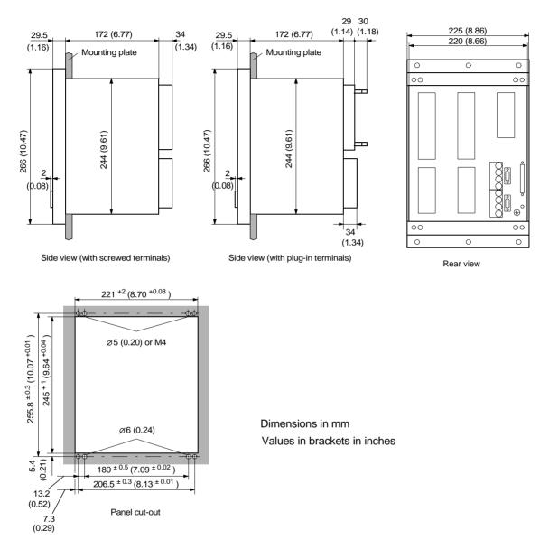
Figure 10-8 Dimensions 7SA6 for panel flush mounting or cubicle installation (size  $\frac{1}{2} \times 19^{\circ}$ )
