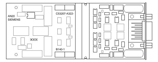
Figure 8-20 Interface module with the analog output AN20
