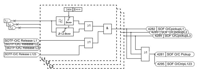
Figure 6-87 Logic diagram of the high current switch on to fault protection
