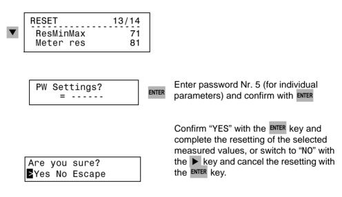
Figure 7-25 Setting of metered values and minimum/maximum values on front panel
