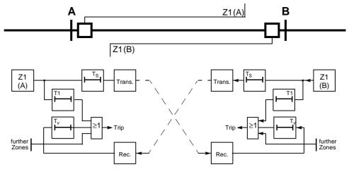
Figure 6-46 Operation scheme of the direct underreach transfer trip method
