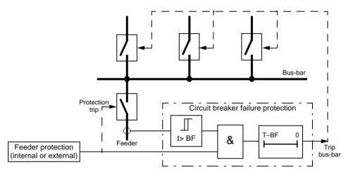
Figure 6-111 Simplified function diagram of circuit breaker failure protection with current flow monitoring
