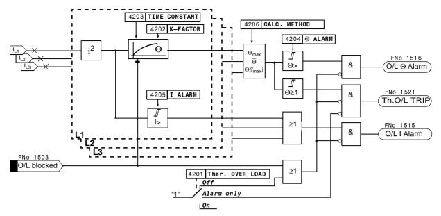
Figure 6-129 Logic diagram of the thermal overload protection
