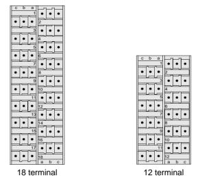
Figure 2-14 Terminal blocks of plug-in terminals for voltage connections - rear view
