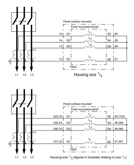
Figure A-20 Current connections to three current transformers with a star-point connection for earth current (residual  $3I_0$  neutral current), normal circuit layout — appropriate for all networks
