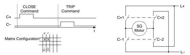
Figure 5-11 Double command motor control (anti-clockwise rotation / clockwise rotation) via two power relays with two contacts each
