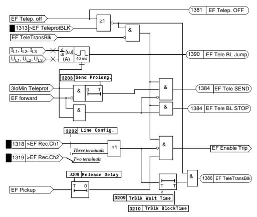
Figure 6-76 Logic diagram of the blocking scheme (one line end)
