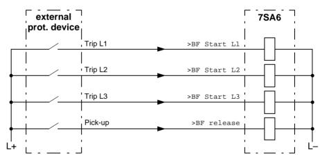
Figure 6-117 Breaker failure protection with phase segregated initiation — example for initiation by an external protection device with release by a fault detection signal
