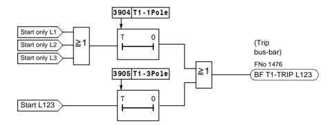
Figure 6-121 Single-stage breaker failure protection with different delay timers
