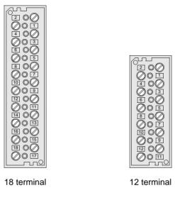
Figure 2-9 Connection plug module with screw terminals for voltage connections — rear view
