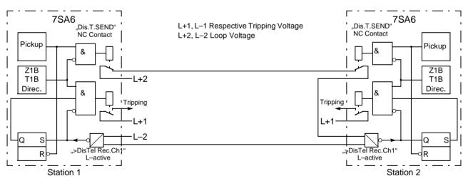
Figure 6-56 Pilot wire protection — principle
