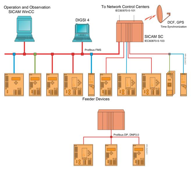
Figure 4-1 Integration of feeder devices in the SICAM substation control system — example
