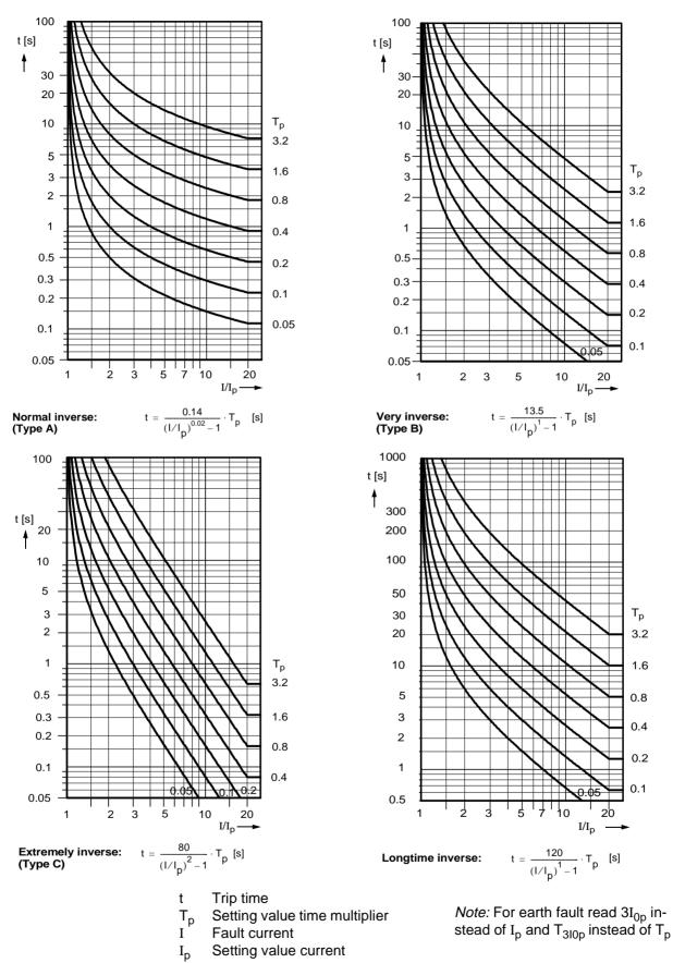
Figure 10-1 Trip time characteristics of inverse time overcurrent protection, acc. IEC (phases and earth)
