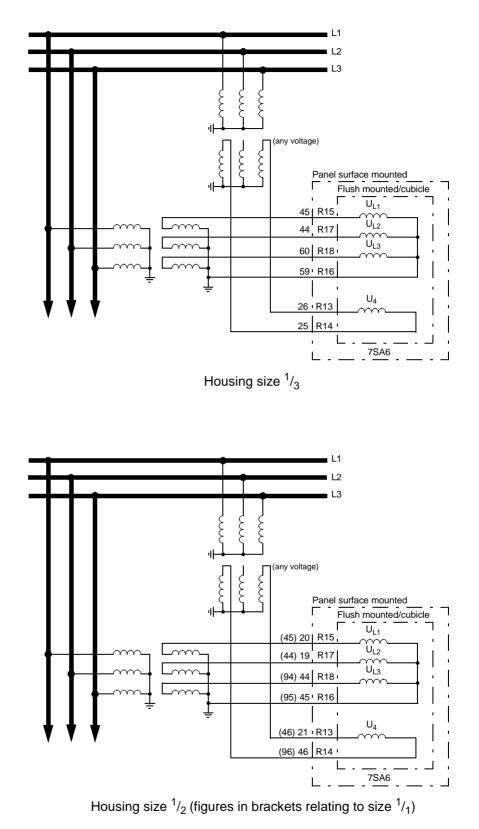
Figure A-27 Voltage connections to three Wye-connected voltage transformers and additionally to any phase-to-phase voltage (for overvoltage protection and/or synchronism check)
