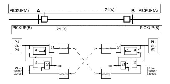
Figure 6-49 Operation scheme of the directional comparison pickup
