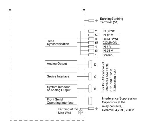
Figure A-12 General Diagram 7SA6\*2\*-\*E (Panel Surface Mounting)
