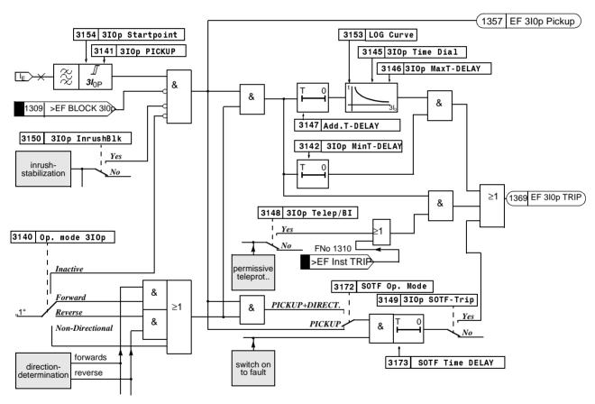
Figure 6-63 Logic diagram of the 3I<sub>0P</sub>-stage for the inverse logarithmic curve
