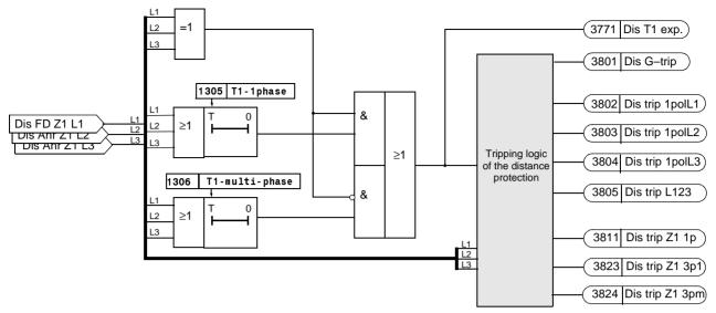
Figure 6-34 Tripping logic for the 1st Zone
