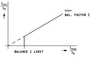
Figure 6-131 Current symmetry monitoring
