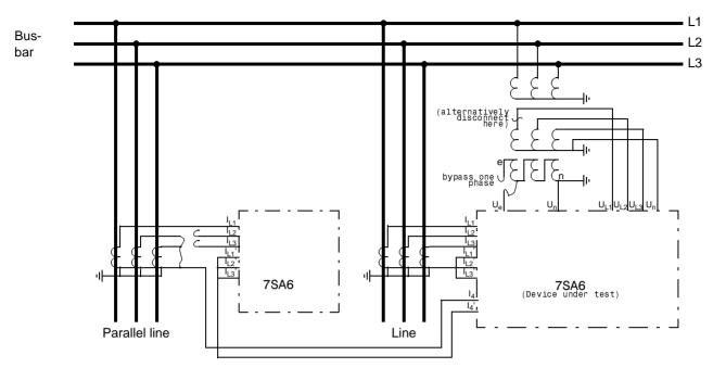
Figure 8-26 Polarity check of I<sub>4</sub>, example with earth current of a parallel line
