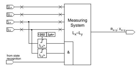
Figure 6-23 Logic of the phase-phase measuring system
