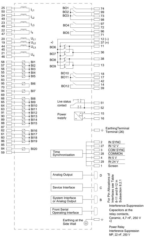
Figure A-11 General Diagram 7SA6\*1\*-\*F (Panel Surface Mounting)
