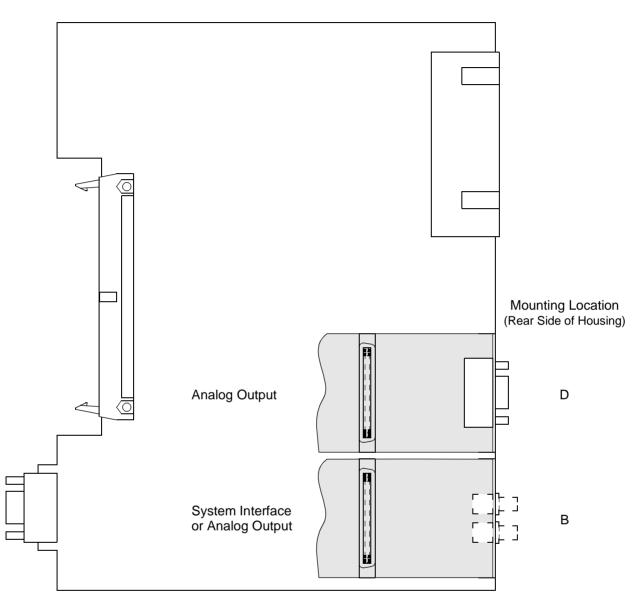
Figure 8-17 Processor printed circuit board C–CPU–2 with interface modules
