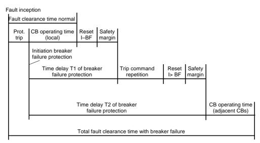
Figure 6-127 Time sequence example for normal clearance of a fault, and with circuit breaker failure, using two-stage breaker failure protection
