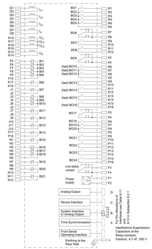
Figure A-5 General Diagram 7SA6\*2\*--\*A/J (panel flush mounted or cubicle mounted)
