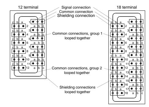
Figure 2-40 Schematic diagram of the plug-in terminal blocks
