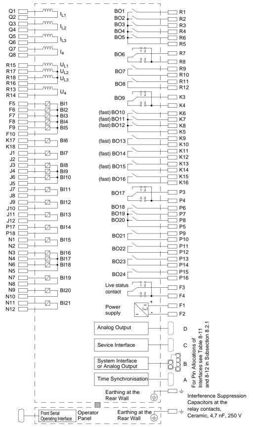
Figure A-17 General Diagram 7SA642\*-\*A/J (Mounting with detached operator panel)
