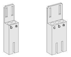
Figure 2-17 2-pin connector and 3-pin connector
