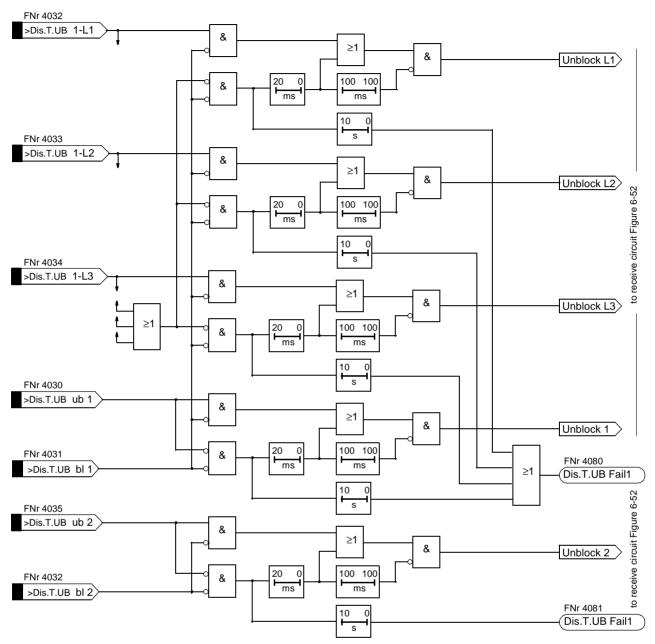
Figure 6-53 Unblock–logic
