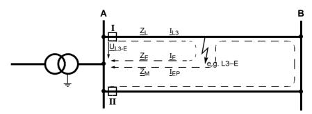
Figure 6-27 Earth fault on a double circuit line
