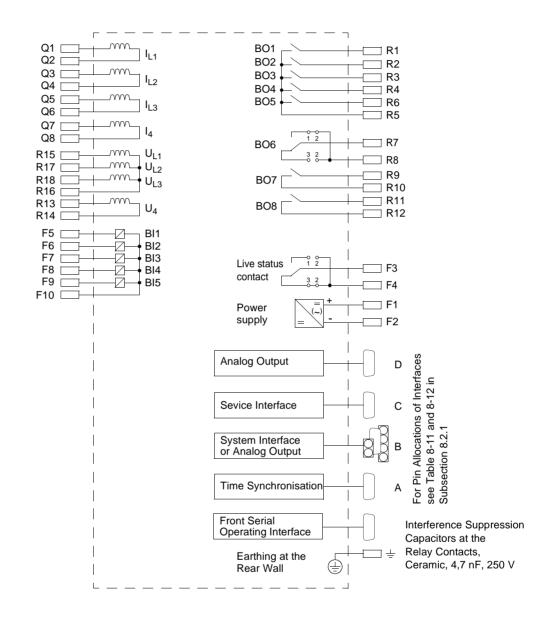
Figure A-1 General Diagram 7SA610\*-\*A/J (panel flush mounted or cubicle mounted)
