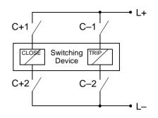
Figure 5-9 Double command with double contacts (with 4 relays)
