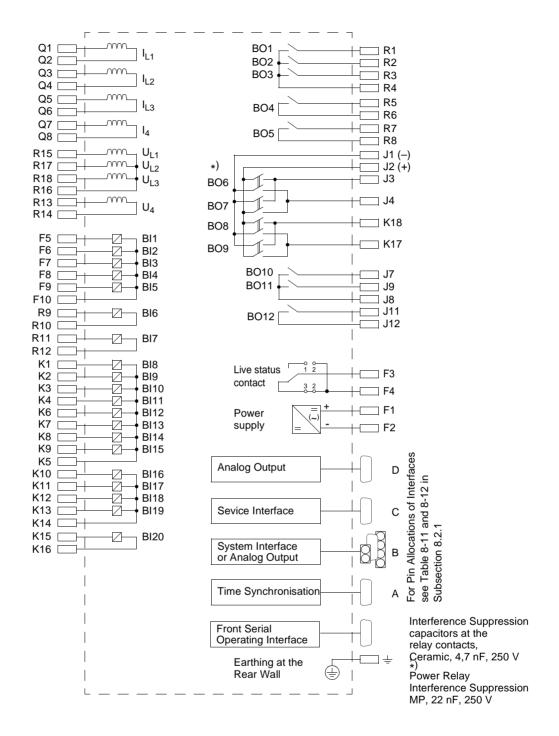
Figure A-4 General Diagram 7SA6\*1\*-\*B/K (panel flush mounted or cubicle mounted)
