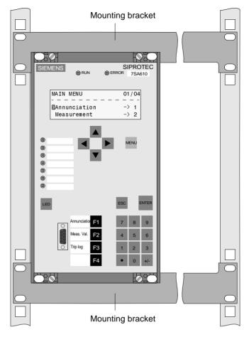
Figure 8-4 Installing a 7SA610 with a four-line display in a rack or cubicle (housing width  $1/_3$  of 19 inch rack) as an example
