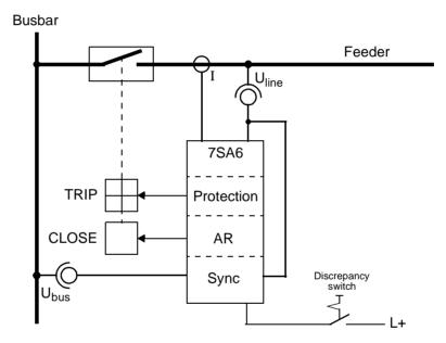
Figure 6-103 Synchronism check on closing
