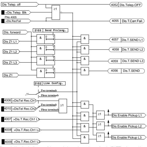
Figure 6-43 Logic diagram of the permissive underreach transfer trip (PUTT) scheme with pick-up (one line end)
