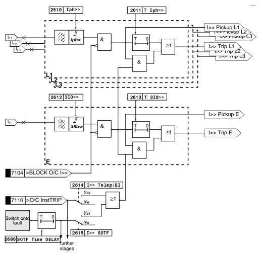
Figure 6-83 Logic diagram of the I>>-stage
