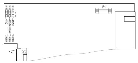
Figure 9-7 Power supply mini-fuse CPU board
