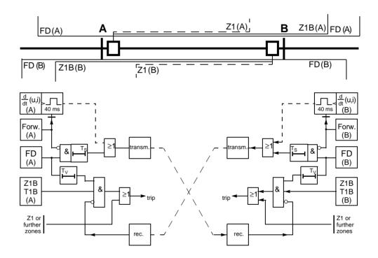
Figure 6-54 Operation scheme of the blocking method
