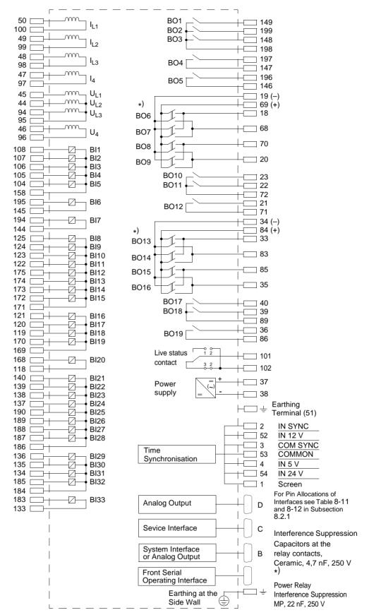
Figure A-14 General Diagram 7SA6\*2\*-\*G (Panel Surface Mounting)
