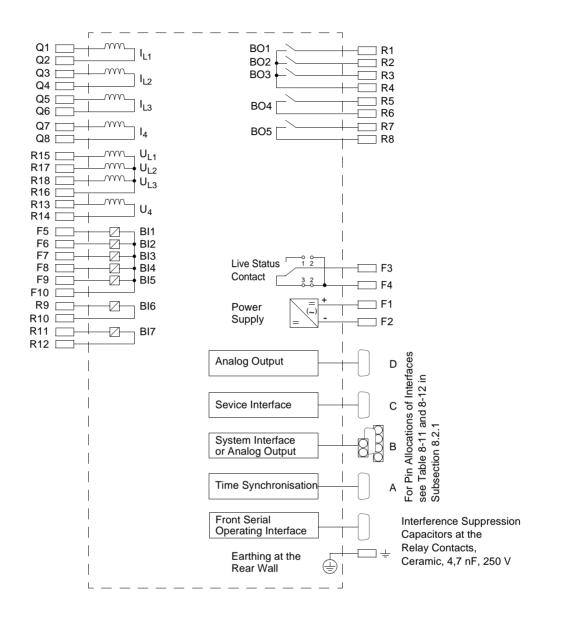
Figure A-2 General Diagram 7SA610\*-\*B/K (panel flush mounted or cubicle mounted)
