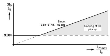
Figure 6-65 Phase current stabilization
