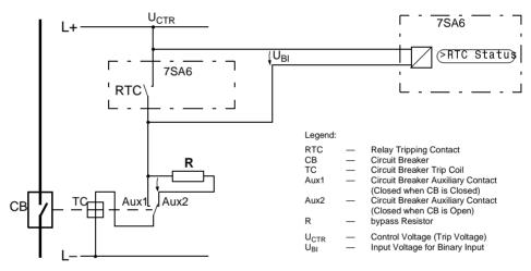
Figure 8-7 Trip circuit supervision with one binary input
