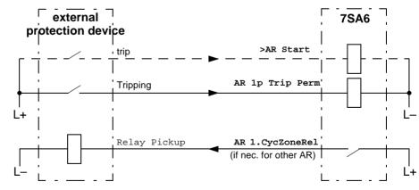
Figure 6-100 Connection example with external protection device for 3-pole reclosure; AR control mode = *with TRIP*
