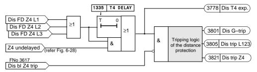
Figure 6-37 Tripping logic for the 4th and 5th Zone, shown is zone Z4
