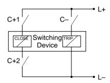
Figure 5-10 Double command with double and single contacts (with 3 relays)
