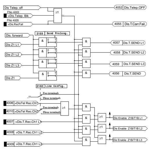
Figure 6-45 Logic diagram of the permissive underreach transfer trip (PUTT) scheme using Z1B (one line end)
