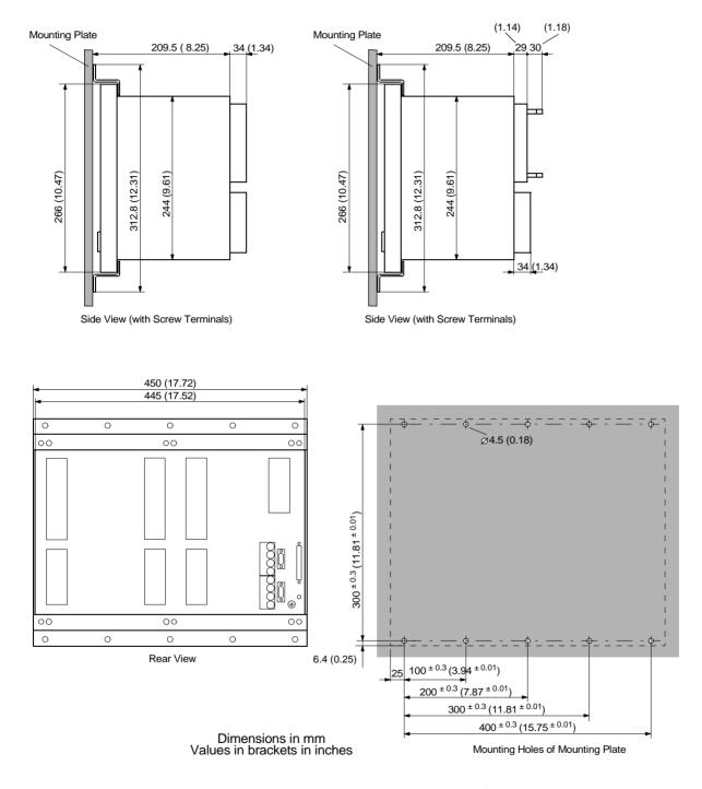
Figure 10-14 Dimensions 7SA6 for mounting with detached operator panel (size  $\frac{1}{1} \times 19$ ")
