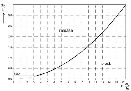
Figure 6-16 Characteristic of the  $I_0/I_2$ -stage
