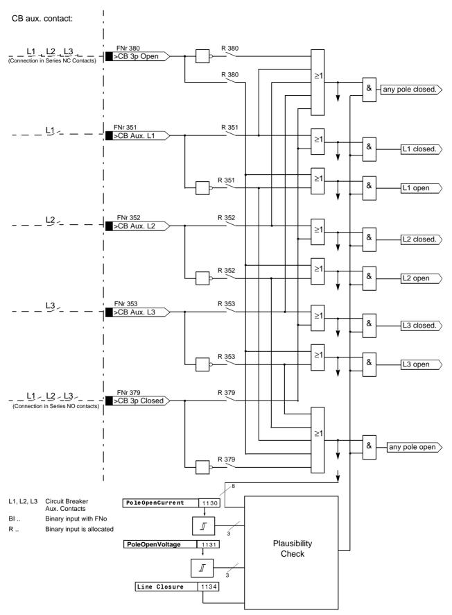
Figure 6-141 Circuit breaker position logic
