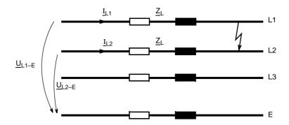
Figure 6-22 Short circuit of a phase-phase loop
