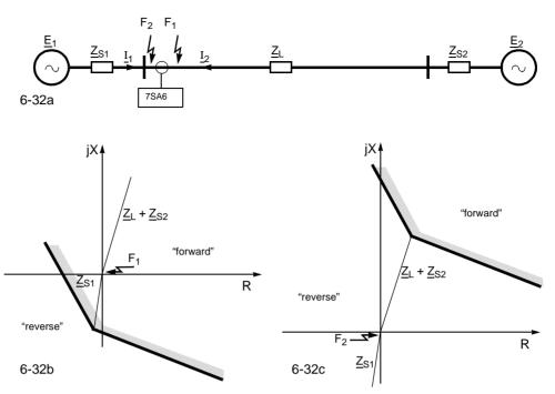
Figure 6-32 Directional characteristic with quadrature or memorized voltages
