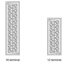
Figure 2-33 Connection plug module with screw terminals for voltage connections — rear view
