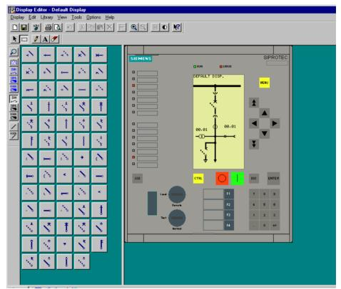
Figure 5-48 Default Display in Normal Size View
