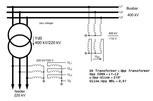
Figure 6-9 Busbar voltage, measured across a power transformer
