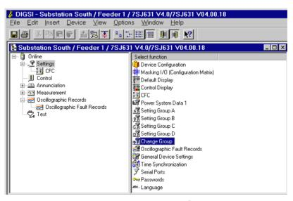
Figure 7-36 Function selection window in DIGSI<sup>®</sup> 4 – example
