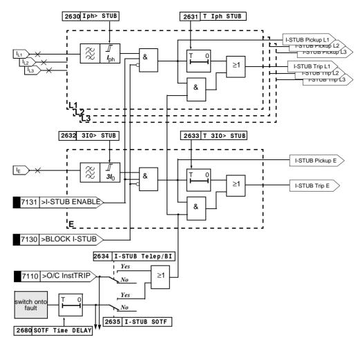
Figure 6-86 Logic diagram of the stub protection
