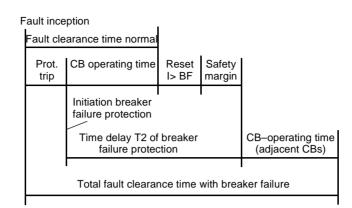
Figure 6-128 Time sequence example for normal clearance of a fault, and with circuit breaker failure, using single-stage breaker failure protection
