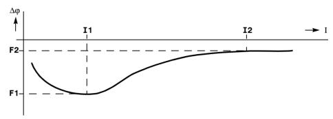
Figure 6-92 Settings for the phase angle correction
