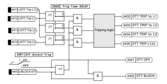
Figure 6-82 Logic diagram of the local external tripping
