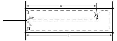
Figure 6-12 reach with Parallel Line Compensation at II
