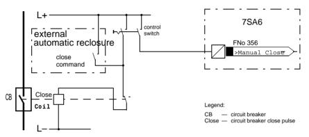
Figure 6-140 Manual closure with external automatic reclosure
