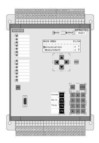
Figure 2-22 Front view of a 7SA61, housing size 1/2, for panel flush mounting without optical communication interfaces
