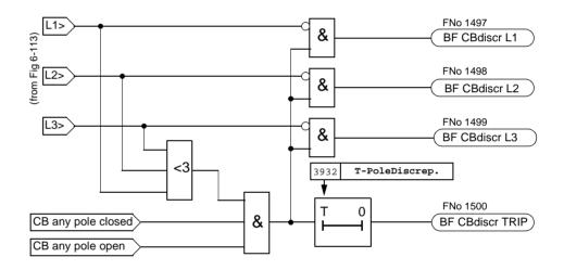
Figure 6-126 Function block diagram of pole discrepancy supervision
