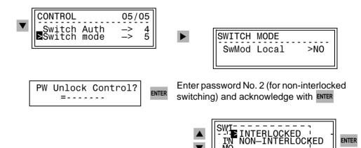
Figure 7-56 Operating Menu for Switching Mode Using Front Panel
