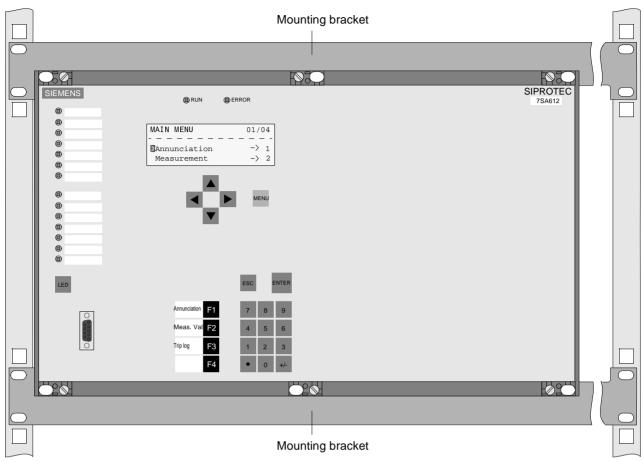
Figure 8-6 Installing a 7SA612 with a four-line display in a rack or cubicle (housing width 1/1 of 19 inch rack) as an example
