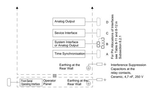
Figure A-18 General Diagram 7SA642\*-\*B/K (Mounting with detached operator panel)
