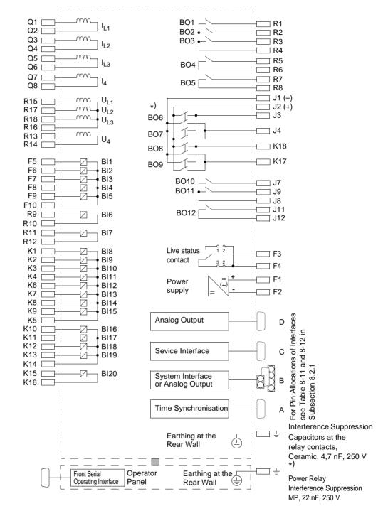
Figure A-16 General Diagram 7SA641\*-\*B/K (Mounting with detached operator panel)
