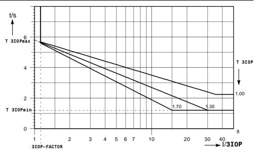
Logarithmic inverse:  $t = T_{3I0Pmax} - T_{3I0P} \cdot ln(I/3I0P)$
