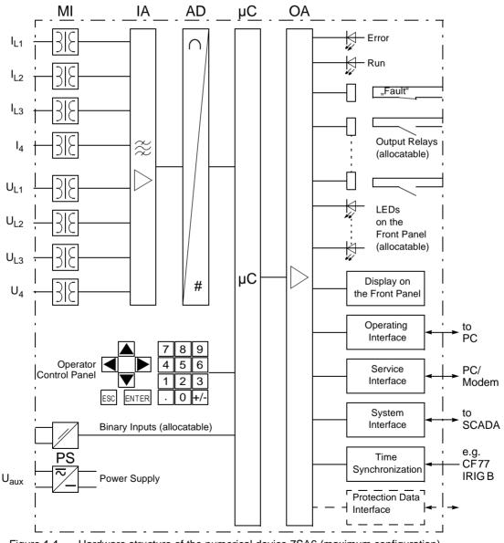
Figure 1-1 Hardware structure of the numerical device 7SA6 (maximum configuration)
