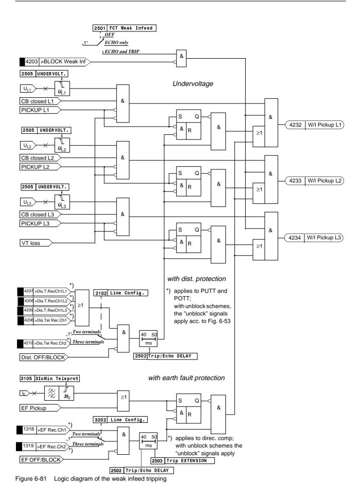
To avoid a faulty pick up of the weak infeed function following tripping of the line and reset of the fault detection, the function cannot pick up any more once a fault detection in the affected phase was present (RS flip-flop in Figure 6-81).
