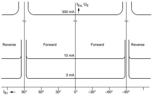
Figure 6-89 Directional earth fault measurement characteristic in a resonant-earthed system
