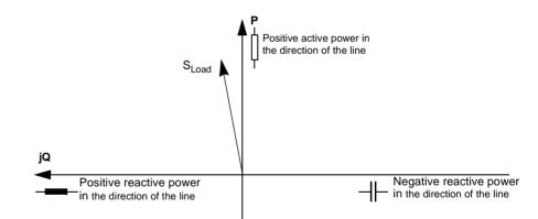
Figure 8-23 Complex (apparent) power
