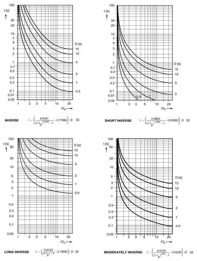
Figure 10-2 Trip time characteristics of inverse time overcurrent protection, acc. ANSI/IEEE, (phases and earth)
