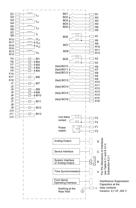
Figure A-3 General Diagram 7SA6\*1\*-\*A/J (panel flush mounted or cubicle mounted)
