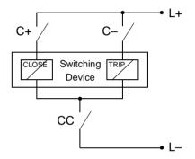
Figure 5-7 Double command with single contacts plus common contact
