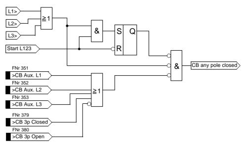
Figure 6-115 Creation process of signal "CB any pole closed"
