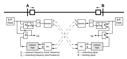
Figure 6-73 Operation scheme of the directional unblocking method
