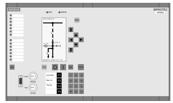
Figure 2-5 Front view of a 7SA63, housing size <sup>1</sup>/<sub>1</sub>, for panel flush mounting or cubicle mounting
