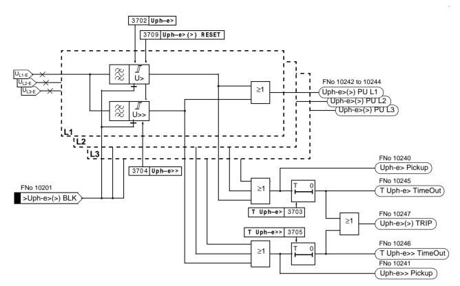
Figure 6-105 Logic diagram of the overvoltage protection for phase voltages
