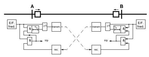
Figure 6-71 Operation scheme of the directional comparison method
