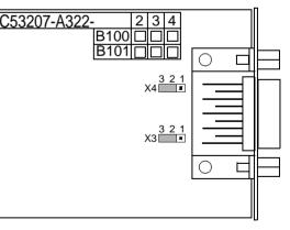
Figure 8-19 Location of the jumpers for the configuration of terminating resistors of the Profibus interface
