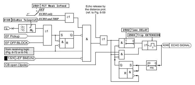
Figure 6-78 Logic diagram of the echo function for the earth fault protection with teleprotection
