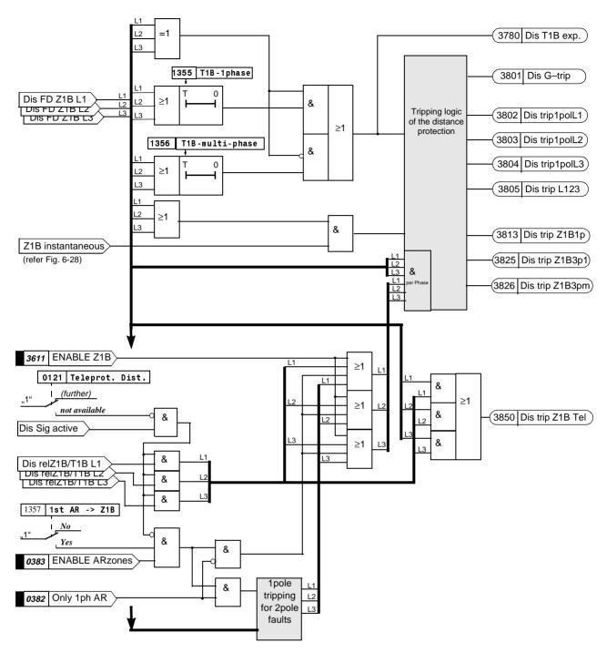
Figure 6-38 Tripping logic for the controlled zone Z1B
