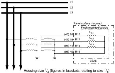
Figure A-24 Voltage connections to three Wye-connected voltage transformers (normal circuit layout)
