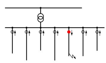
Figure 6-90 Faulted line location in radial network
