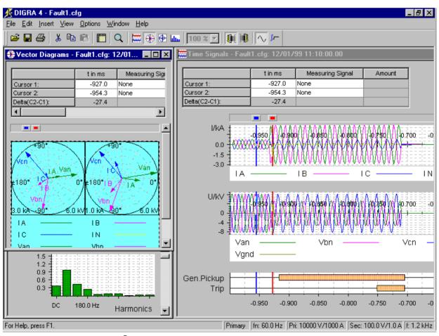
Figure 4-8 DIGRA<sup>®</sup> 4 graphical representations of the waveform data — view examples
