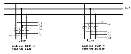
Figure 6-8 Current transformer polarity
