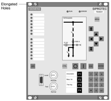
Figure 8-2 Panel mounting of a 7SA631 with graphic display (housing width  $1/_2$ ) as an example
