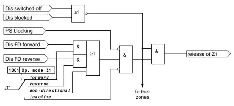
Figure 6-33 Release logic for a zone (example for Z1)
