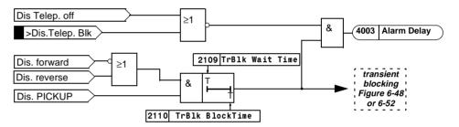
Figure 6-58 Transient blocking with POTT and Unblocking schemes
