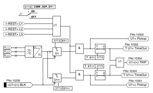
Figure 6-109 Logic diagram of the undervoltage protection for positive sequence voltage system
