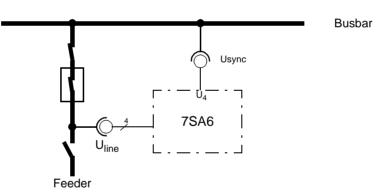
Figure 8-24 Measuring voltages for synchro-check
