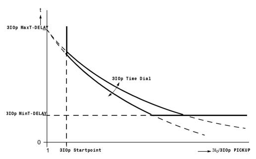
Figure 6-68 Setting parameter characteristics in the logarithmic–inverse curve
