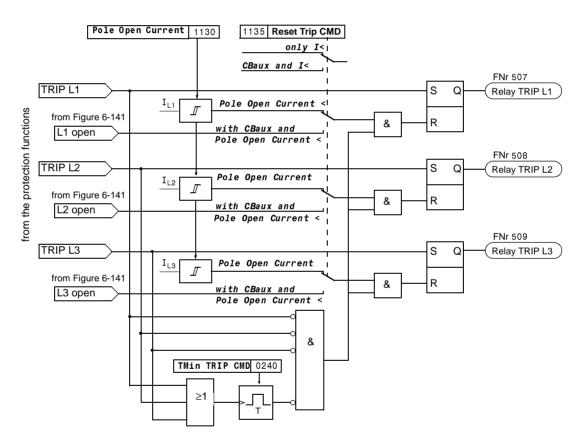
Figure 6-142 Latching and reset of the trip command
