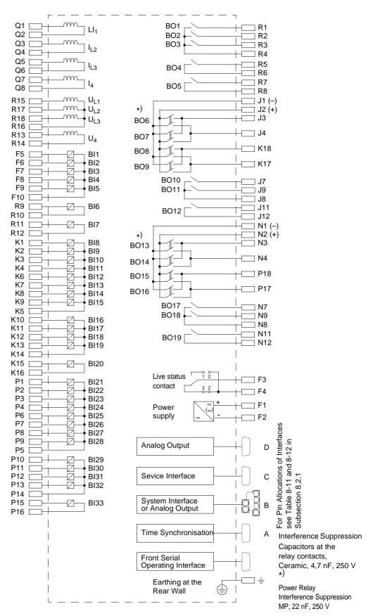
Figure A-7 General Diagram 7SA6\*2\*--\*C/L (panel flush mounted or cubicle mounted)
