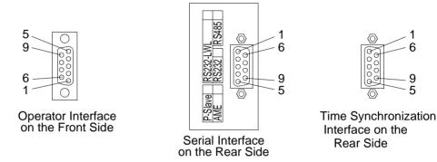
Figure 2-43 9 pin D-subminiature connectors
