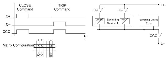
Figure 5-8 Double command with single output common to a bus
