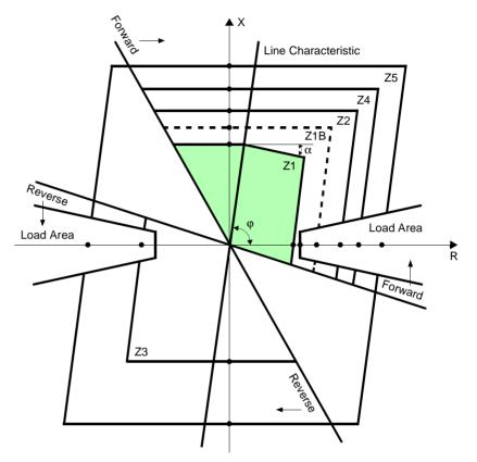
Figure 6-29 Polygonal characteristic
