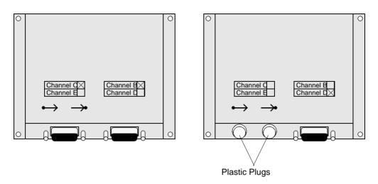
Figure 2-29 Inclined housing with 9-pin DSUB socket
