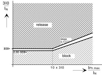
Figure 6-15 Earth current stage: pick-up characteristic — example
