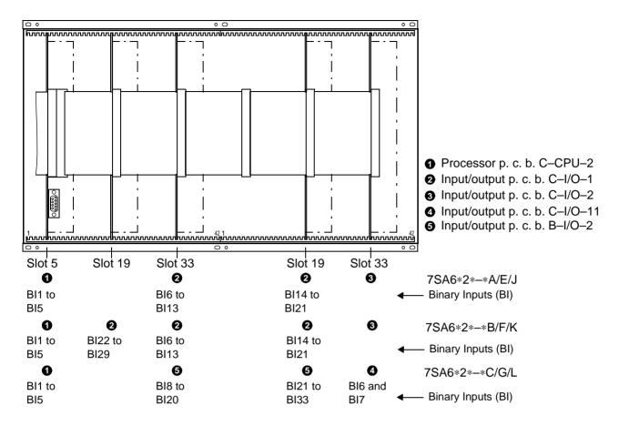
Figure 8-10 Front view of the device with housing size 1/2 after removal of the front cover (simplified and scaled down).
