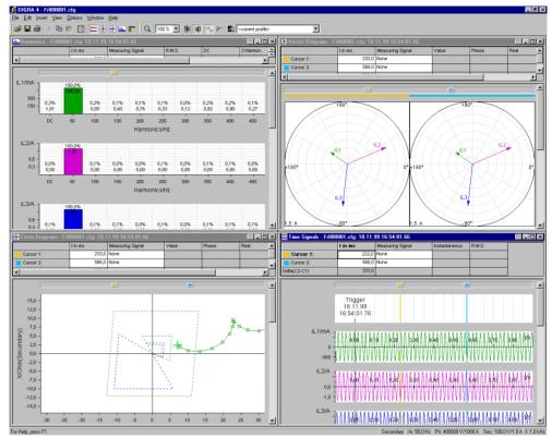
Selection takes place using the menu bar (**View**), or clicking in the symbol bar above the represented switching fields. Figure 7-27 shows all four views simultaneously.
