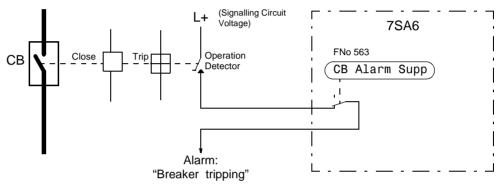
Figure 6-144 Breaker tripping alarm suppression
