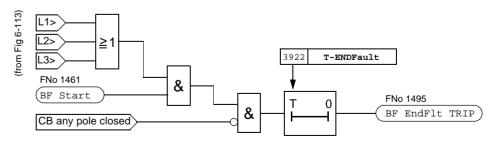
Figure 6-125 Function block diagram of end fault protection
