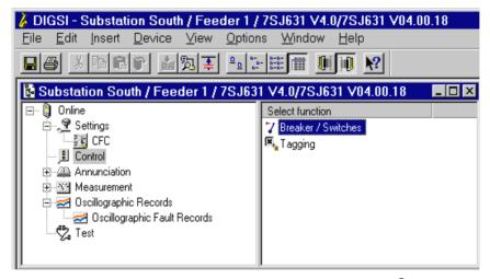
Figure 7-48 Window for Control of Operating Resources in DIGSI<sup>®</sup> 4 - (example)
