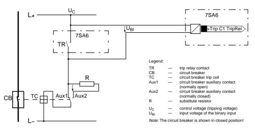
Figure 6-136 Operating principle of the trip circuit supervision with one binary input
