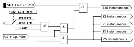
Figure 6-28 Circuit breaker closure onto a fault
