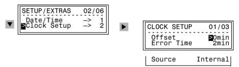
Figure 7-30 Date and time settings from the front panel
