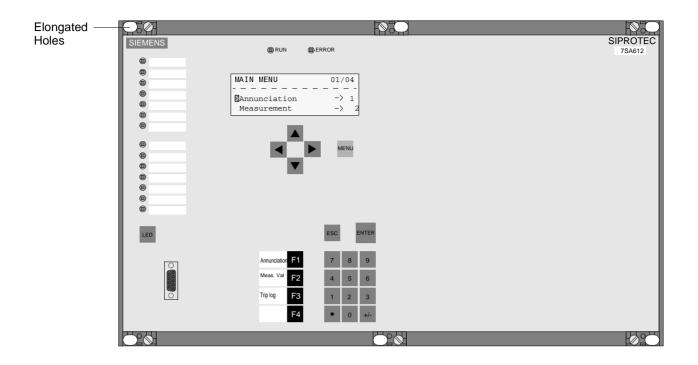
Figure 8-3 Panel mounting of a 7SA612 with a four-line display (housing width 1/1) as an example
