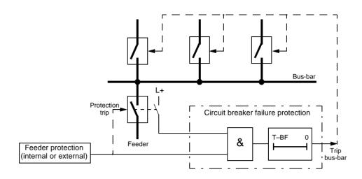
Figure 6-112 Simplified function diagram of circuit breaker failure protection controlled by circuit breaker auxiliary contact
