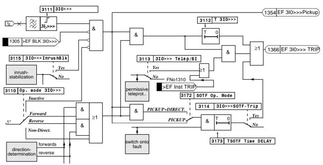
Figure 6-61 Logic diagram of the 3I<sub>0</sub>>>>-stage
