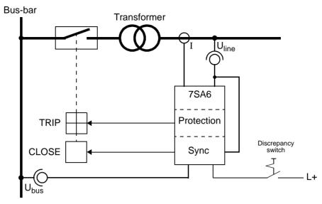
Figure 6-104 Synchronism check across a transformer
