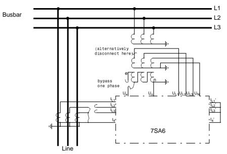
Figure 8-25 Polarity testing for I<sub>4</sub>, example with current transformers configured in a Holmgreen-connection
