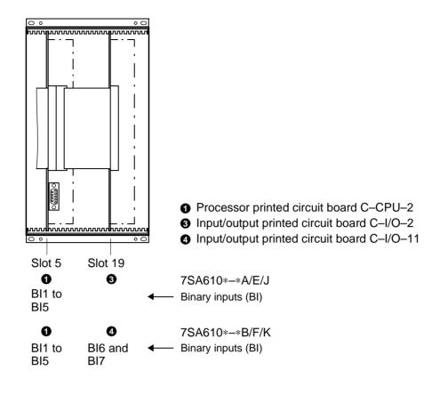
Figure 8-8 Front view of device of housing size 1/3 after removal of the front cover (simplified and scaled down)
