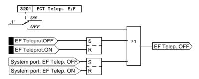
Figure 6-70 Switching on and off of the signal transmission logic
