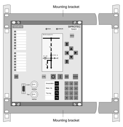
Figure 8-5 Installing a 7SA631 with graphic display in a rack or cubicle (housing width  $^{1}/_{2}$  of 19 inch rack) as an example
