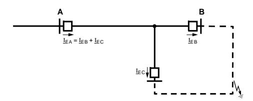
Figure 6-80 Possible unfavourable current distribution on a three terminal line during an external earth fault.
