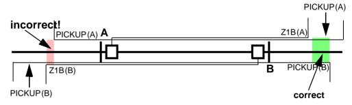
Figure 6-60 Distance protection setting with permissive overreach schemes
