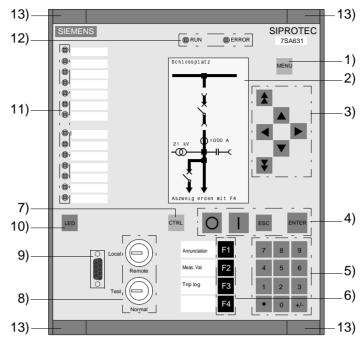
Figure 2-4 Front view of a 7SA63, housing size 1/2, for panel flush mounting or cubicle mounting
