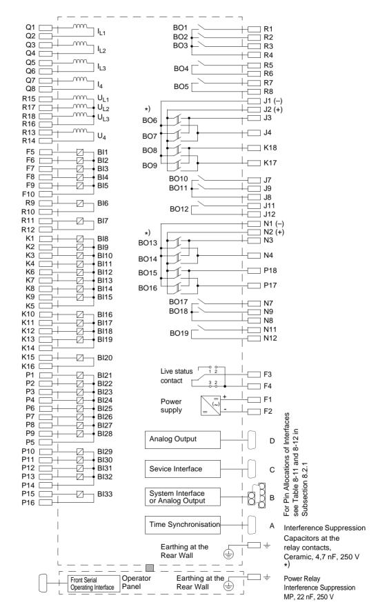
Figure A-19 General Diagram 7SA642\*-\*C/L (Mounting with detached operator panel)
