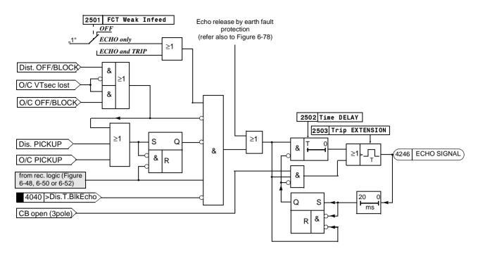
Figure 6-59 Logic diagram of the echo function with distance protection teleprotection
