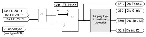
Figure 6-36 Tripping logic for the 3rd Zone
