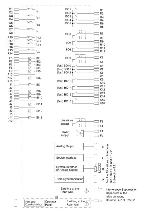
Figure A-15 General Diagram 7SA641\*-\*A/J (Mounting with detached operator panel)
