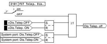
Figure 6-41 Switching on and off of the teleprotection
