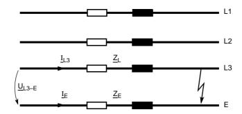
Figure 6-24 Short circuit of a phase-earth loop
