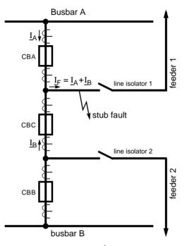
Figure 6-85 Stub fault at an 1<sup>1</sup>/<sub>2</sub>-circuit breaker arrangement
