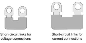
Figure 2-36 Short-circuit links for voltage connections and current connections
