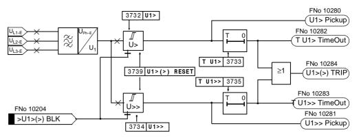
Figure 6-106 Logic diagram of the overvoltage protection for the positive sequence voltage system
