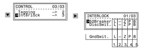
Figure 7-53 Example of Interlocking Conditions for Switching Equipment, Front Panel
