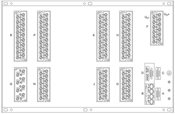
Figure 2-8 Rear view of a 7SA6, housing size <sup>1</sup>/<sub>1</sub> (terminal arrangement example only)
