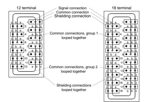
Figure 2-16 Schematic diagram of the plug-in terminal blocks
