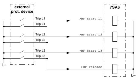
Figure 6-118 Breaker failure protection with phase segregated initiation — example for initiation by an external protection device with release by a separate set of trip contacts
