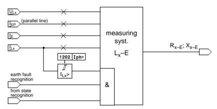
Figure 6-25 Logic of the phase-earth measuring system
