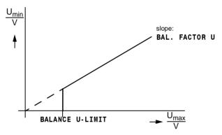
Figure 6-132 Voltage symmetry monitoring
