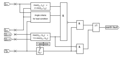
Figure 6-18 Earth fault recognition during single-pole open condition
