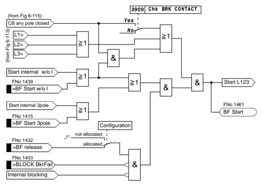
Figure 6-116 Breaker failure protection with common phase initiation
