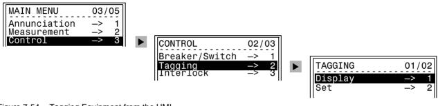
Figure 7-54 Tagging Equipment from the HMI
