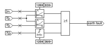
Figure 6-17 Logic of the earth fault recognition
