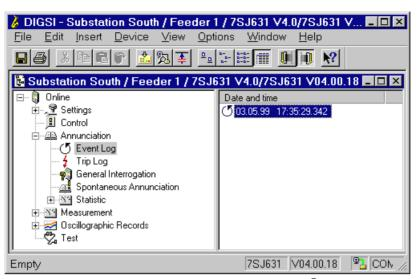
Figure 7-4 Selection of operational messages in DIGSI<sup>®</sup> 4
