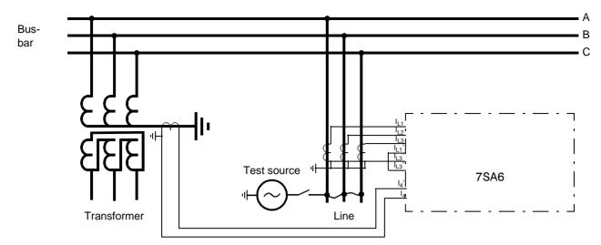
Figure 8-27 Polarity check of I<sub>4</sub>, example with earth current from a power transformer star-point
