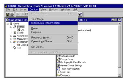
Figure 7-40 Example: Transfer Block Activated in DIGSI<sup>®</sup> 4
