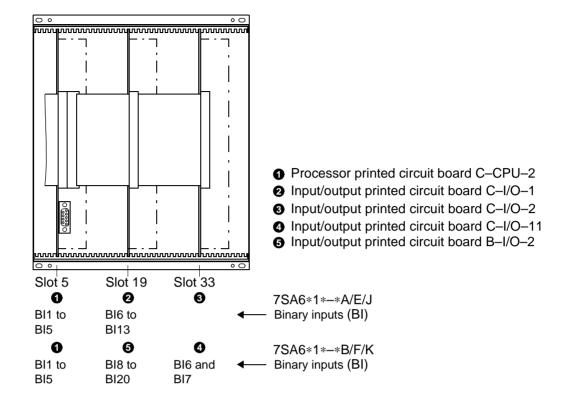
Figure 8-9 Front view of the device with housing size <sup>1</sup>/<sub>2</sub> after removal of the front cover (simplified and scaled down)
