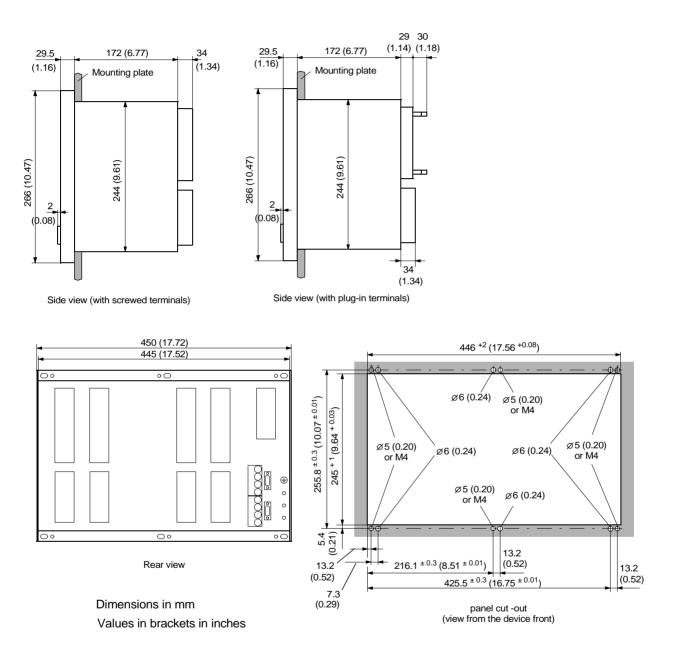
Figure 10-9 Dimensions 7SA6 for panel flush mounting or cubicle installation (size  $\frac{1}{1} \times 19$ ")
