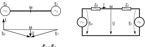
$$\underline{I} = \frac{\underline{E}_1 - \underline{E}_2}{\underline{Z}_1 + \underline{Z}_2}$$
