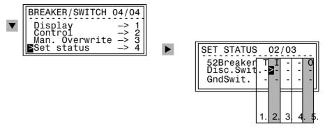
Figure 7-52 Set Status at the Front Panel (example)
