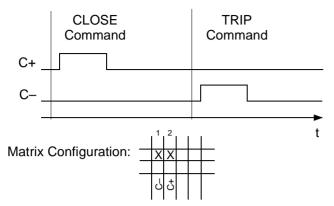
Figure 5-6 Double command with single contacts
