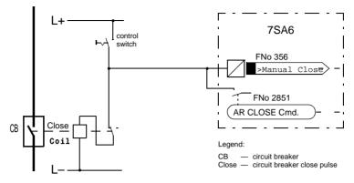
Figure 6-139 Manual closure with internal automatic reclosure
