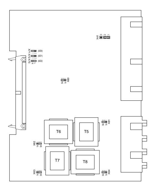
Figure 8-14 The input/output board C-I/O–2 with the jumpers necessary for the setting check
