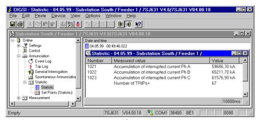
Figure 7-16 List of statistic values in DIGSI<sup>®</sup> 4 — example
