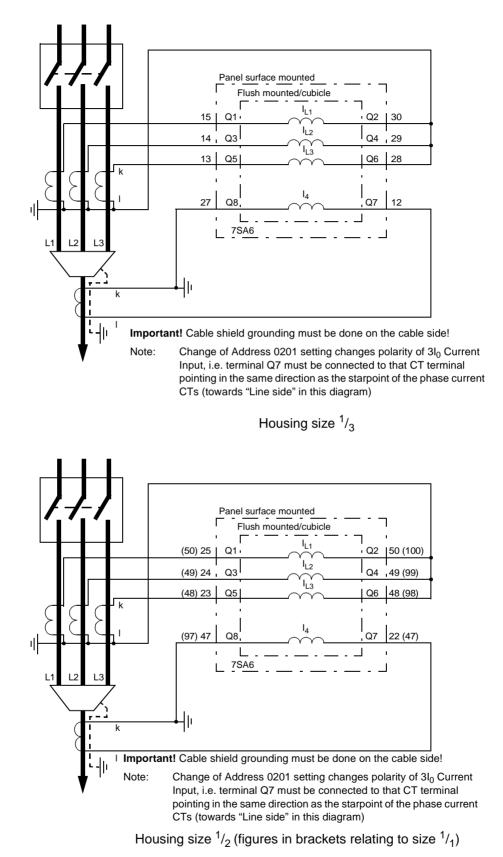
Figure A-21 Current connections to three current transformers with separate earth current transformer (summation current transformer or cable core balance current transformer)
