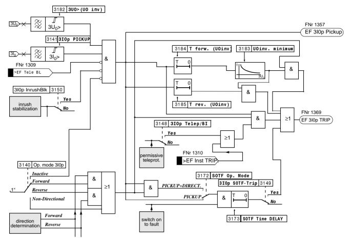
Figure 6-64 Directional zero voltage time protection with non-directional back-up stage
