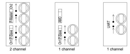
Figure 2-18 Optical communication interfaces with protective caps
