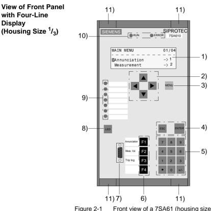
Figure 2-1 Front view of a 7SA61 (housing size 1/3) for panel flush mounting or cubicle mounting
