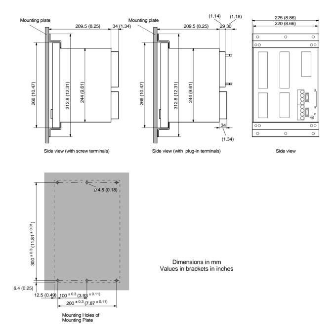
Figure 10-13 Dimensions 7SA6 for mounting with detached operator panel (size  $\frac{1}{2} \times 19$ ")
