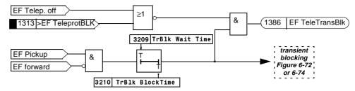
Figure 6-77 Transient blocking for a directional comparison and directional unblocking schemes
