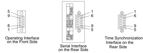
Figure 2-19 9 pin D-subminiature connectors
