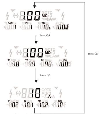
Figure 2 - The result of a polarity index test (PI)
