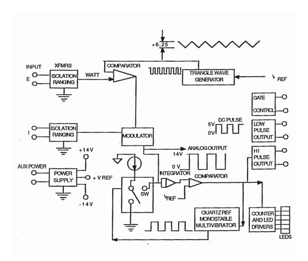
Figure 3.1 Simplified Block Diagram -  $SC^{\$}10V$  Operation
