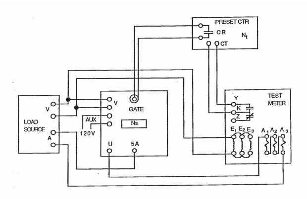
Figure 2.2 Connections and Setup for Testing a Meter Using a Pulse Initiator (KYZ) Output
